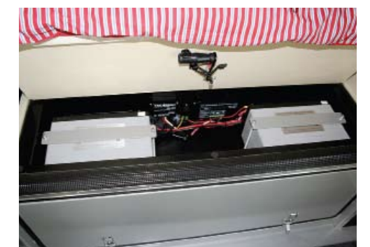
ABOVE One of the advantages of AGM batteries is that they can be mounted on their side, as in this Aussie Swag camper van.
