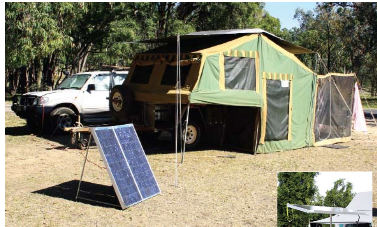
ABOVE By remotely locating the panels, this camper is able to best adapt to the sun's motion in the sky and changing circumstances.
