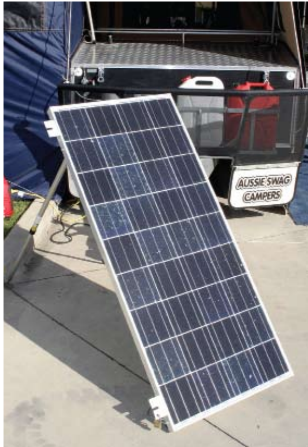
ABOVE No shadows and a clear view towards the sun ensure this solar panel set-up will generate maximum amounts of power.
