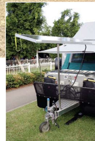
ABOVE One option would be to mount your panel on an arm above the draw bar.
